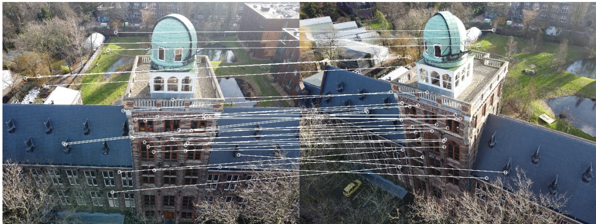
Figure 5 - Finding corresponding features in each overlapping pair of images. These points are called tie points.
