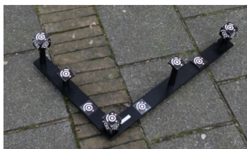
Figure 4 - Control Points Scale Bar to calibrate a camera.
